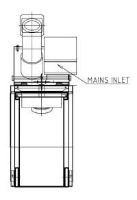
The Evac U 80 glass crusher is a user-friendly solution for the processing of glass. Bottles are manually fed through the feed pipe and the glass pieces are collected in a standard 80-liter wheelie bin. The volume reduction is approximately 80%.
