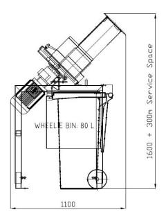
The unit is fitted with a level indicator that automatically stops the crusher when the bin is full. By using different bins it is possible to separate uncolored and colored glass.
